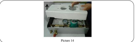
• Open the terminal box, disconnect the power supply connection.
