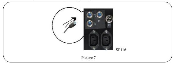
Connect auxiliary heating wire if available. Cable (coffee) for the "L", cable (blue) for "N" line, cable (yellow-green) for the ground wire.
