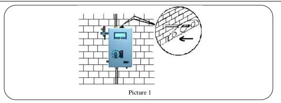
• Drill the holes for dowels, put the dowels into the holes, fixed the solar control system on the wall using fastening screws. The solar control system must be vertically installed. See picture 2.
