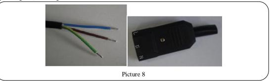
• To connect external circulation pumps or any electromagnetic valves, firstly loose the aviation socket and dismount it as indicated below. Connect the wire to aviation socket, number 1 connects "N" wire (blue color), number 2 connects ground wire (yellow-green color), number 3 connects "L" wire (red color). Reassemble the aviation socket and connect it to the solar control system.
